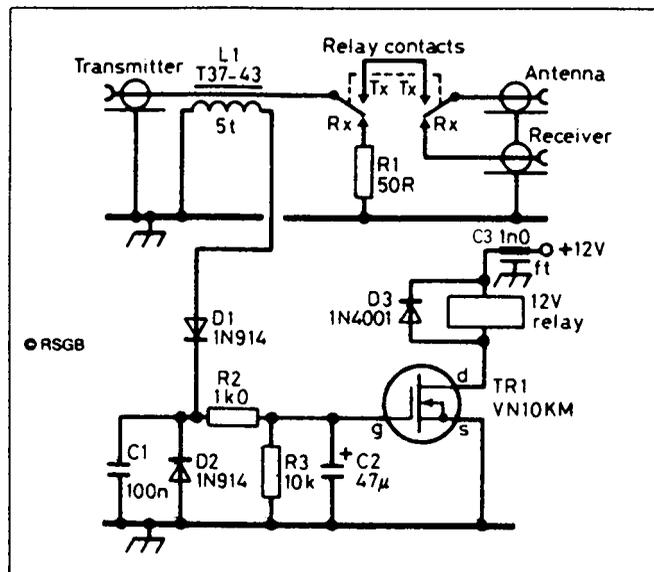
**Figure 1** RF activated relay
