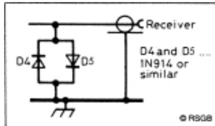
**Figure 3** Receiver input protection
